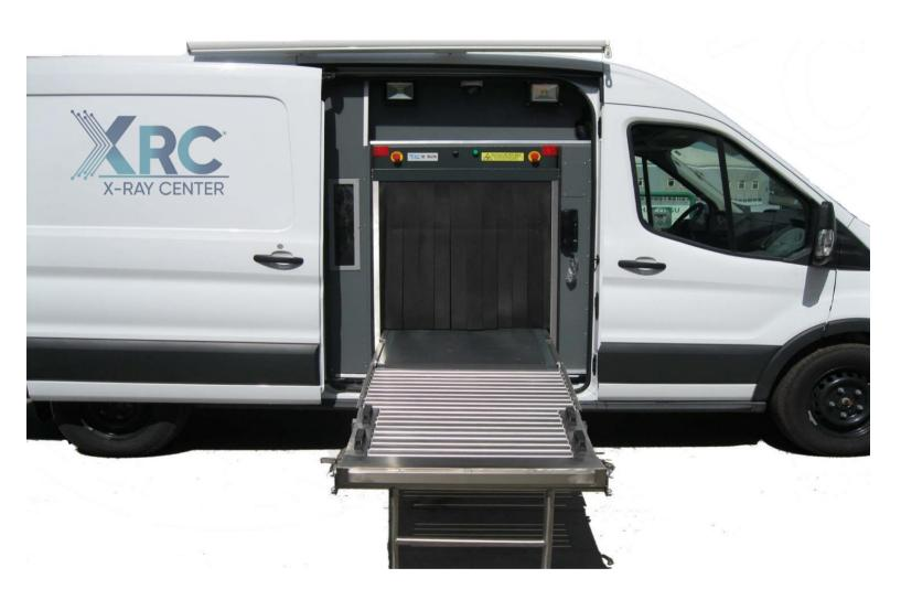
This is the **combine system of x-ray luggage scanner security device and van**. X-ray security device integrated into a van. Due to its mobility, foldable rollers and easy operation, it is frequently used especially at customs gates. It enables easy scanning in places where inspection with fixed devices is not practical. The operator can easily scan the packages from the inside of the vehicle without being exposed to the harsh weather conditions outside the vehicle.
